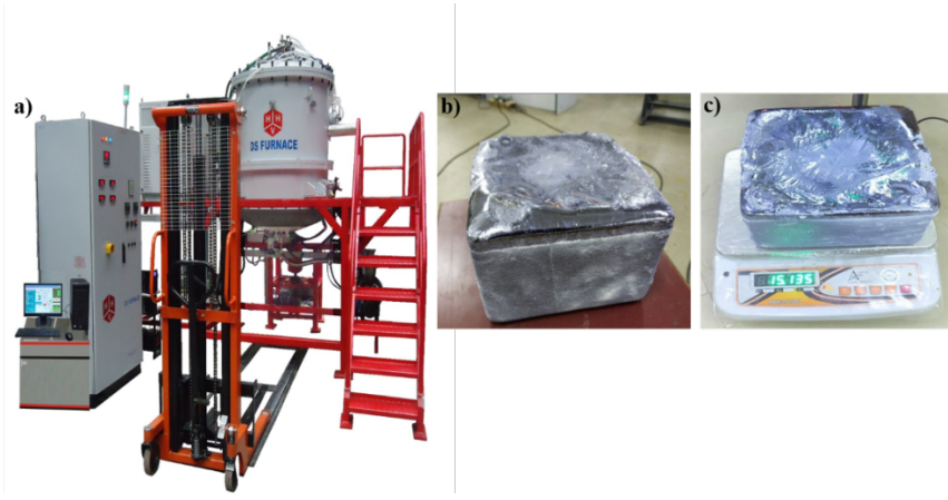
Figure. 1. (a) DS Furnace (b) mc-Silicon ingot (c) Measured ingot weight (15 Kg)
